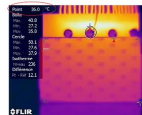
Thermal Image after 5 minutes discharge with 0.508 mm SIGMAclad60 endplate.
