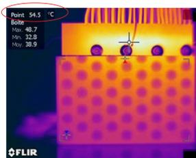
Thermal Image after 5 minutes discharge with 0.250 mm Nickel / 0.250 mm Copper welded assembly endplate
